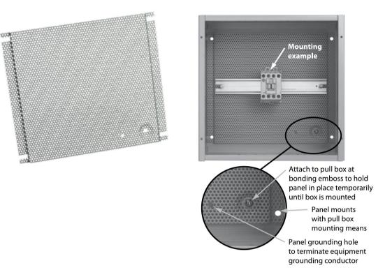
Panel is formed to provide 7/16-in. space off back of pull box for component mounting screw clearance and includes a grounding hole to terminate equipment grounding conductors. Ideal for mounting components that require infrequent access such as control transformers, terminals and contactors.
